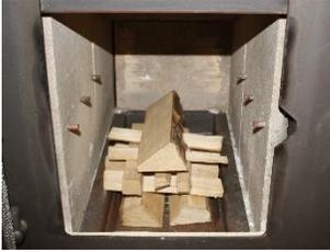
Lay two small wood logs along the length of the firebox base, and place a firelighter / tightly rolled up newspaper on top of them. On top, use wood kindling to create a small lattice structure, before finally placing a small wood log on top.
