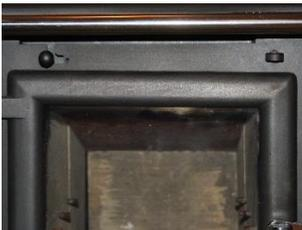
Before lighting your ESSE Ironheart, ensure that the Air Controller is fully open (Pushed to the left) and that the Oven Damper is also fully opened (Fully rotated anticlockwise). If required, the Flue Damper can also be opened, by pushing the lever to the rear of the appliance.
