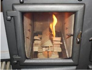
Safely light the firelighter / newspaper and close the door, but leaving it slightly ajar. Once the flames have established on the wood logs, (typically within 3 – 5 minutes), fully close the door and slowly reduce the air volume, by moving the Air Controller to the right. Continue to use the Air Controller to control the fire, until the flames are slowly 'dancing' on top of the wood logs.
